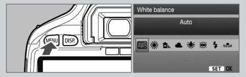
Press the WB button, select the customer white balance on the display and confirm with the "set" button.
