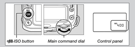
**3.** Set the exposure time to 1/40s. Press the shutter-release briefly until the exposure time appears on the upper control panel. Adjust the value by turning the rear main command dial.
